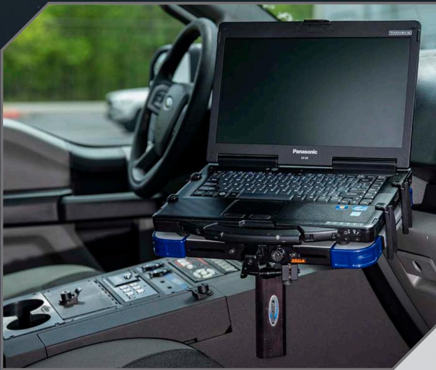
The JOTTO DESK® Console Side Mount (CSM) features No Holes Drilled installation on the passenger side of a compatible equipment console, preserving front passenger side leg room and improving performance. The CSM offers a straight arm which enables you to comfortably use and secure a laptop using the A-MOD or other desktop.
